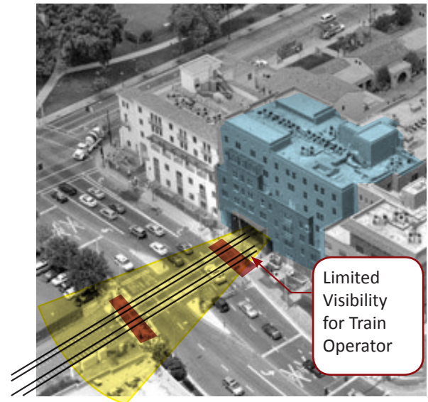
Limited sight-lines for trains approaching street crossings create unsafe conditions.
